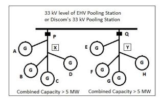
In this case, Generators 'A' to 'D' and 'E' to 'H' are connected to a Pooling Sub-Station of STU or Discom through separate & dedicated feeders having separate inter-connection points at 'P' and 'Q' respectively.
