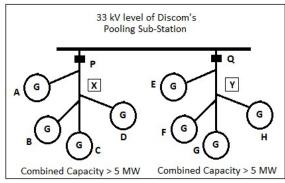
In such case, generators 'A' to 'D' are connected through a common & dedicated feeder 'X' having inter-connection point at 'P', selling power within the State.
