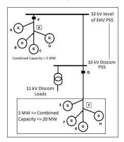
In the said diagram, a group of generators are connected to a 33 kV Discom Pooling Sub-Station connected to a 33kV level of EHV Pooling Sub-Station. In such case, the capacity of generation connected to 33 kV PSS can be aggregated with the capacity of generation connected at EHV Pooling Sub-Station.
