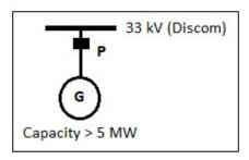
In this case, the Forecasting shall be provided by the QCA at Point 'P'. Scheduling and Accounting shall be done by MSLDC at Point 'P'.
