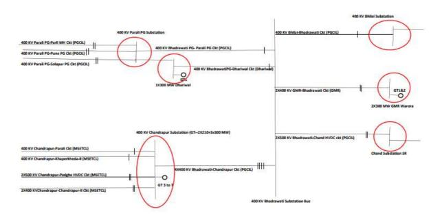
40. It can be seen from the Schematic of transmission system that 400 kV D/c GMR-Bhadrawatickt. Line (proposed under intervening facility) is connected to the
