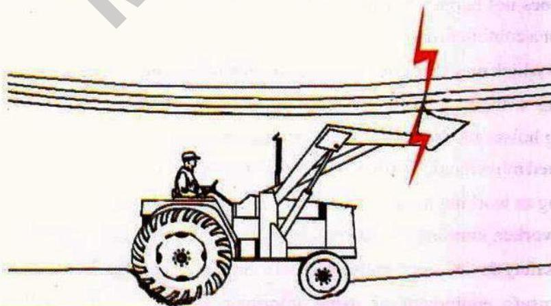
Unsafe working condition results in accident. The boom of Crane moving under electric conductor is seen touching electric line/coming in the vicinity of electric line creating shortcircuit. Conductor may snap or may cause injury to the crane operator.
