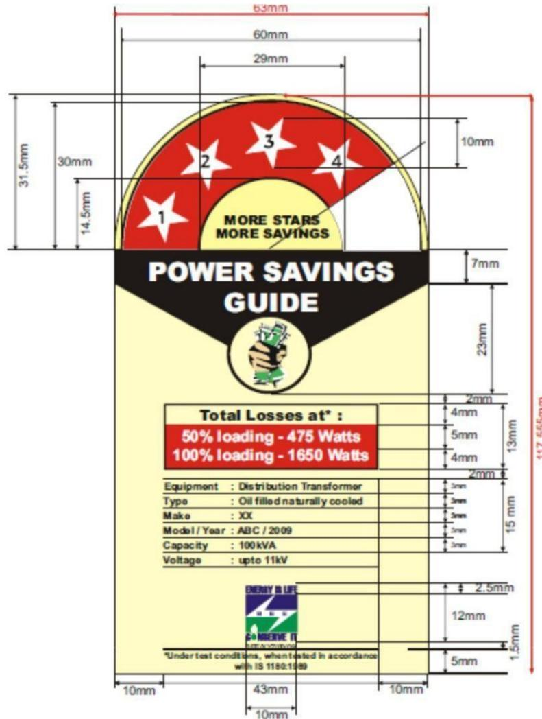
TECHNICAL SPECIFICATION OF 100 KVA, 11/ 0.433 KV and 22/ 0.433 KV, Star 1 (Level-1) THREE PHASE, OIL IMMersed, OUTDOOR, NON SEALEDTYPE DISTRIBUTION TRANSFORMERS WITHOUT CSP FEATURE
