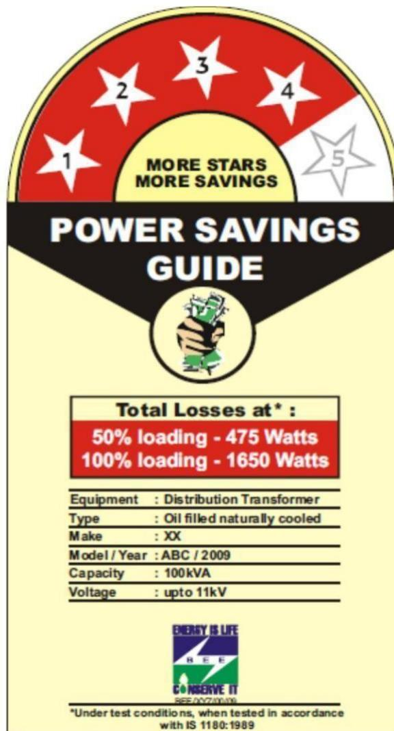
**TECHNICAL SPECIFICATION OF 100 KVA, 11/ 0.433 KV and 22/ 0.433 KV, Star 1 (Level-1) THREE PHASE, OIL IMMERSED, OUTDOOR, NON SEALED TYPE DISTRIBUTION TRANSFORMERS WITHOUT CSP FEATURE**
