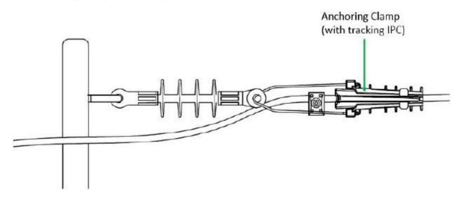
Anchoring with protection against Tracking.
