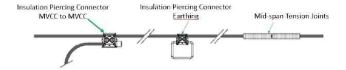
5. Insulation Piercing Connector for Bare to Covered interconnection
